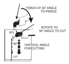
Keep moving while cutting. Cut at a steady speed without pausing. Maintain the cutting speed so that the arc leg is 10° to 20° behind the travel direction.
